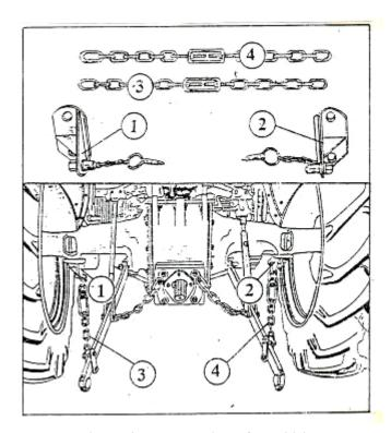
Figure 3 – Installation of stabilizing chains
