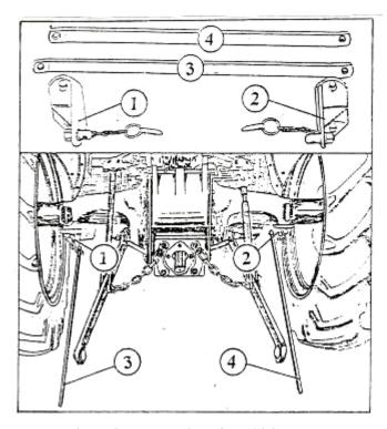
Figure 2 – Installation of stabilizing levers
