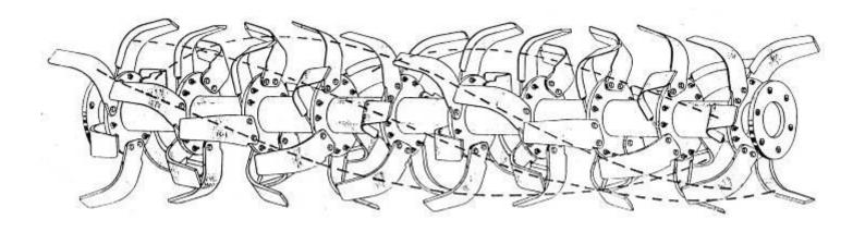
Figure 12. Blades placed in a helical position
