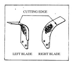
Figure 8. Left and right blade
