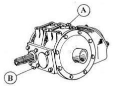
Figure 22. Reduction gear housing
